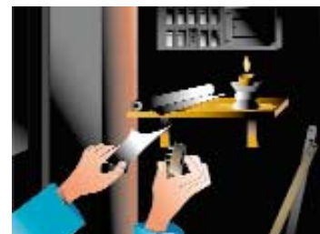
Don't repair fuses with anything other than the correct fuse wire
