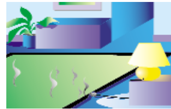
Don't run cables under carpets
